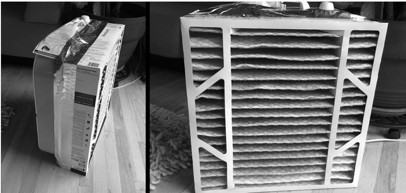
Figure 4: Nettleton’s standalone filter, made of a MERV 13 filter taped onto a floor fan.
